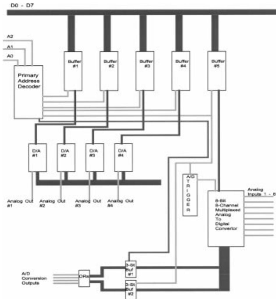
Figure 1. The block diagram of the interface.
