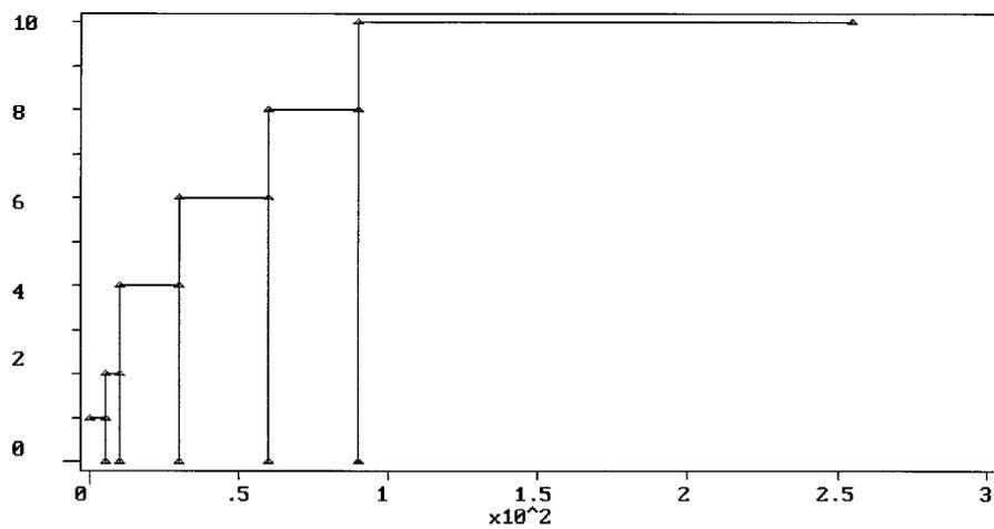
Figure 10. Rate generator transfer function ( $r$  vs.  $E$ )
