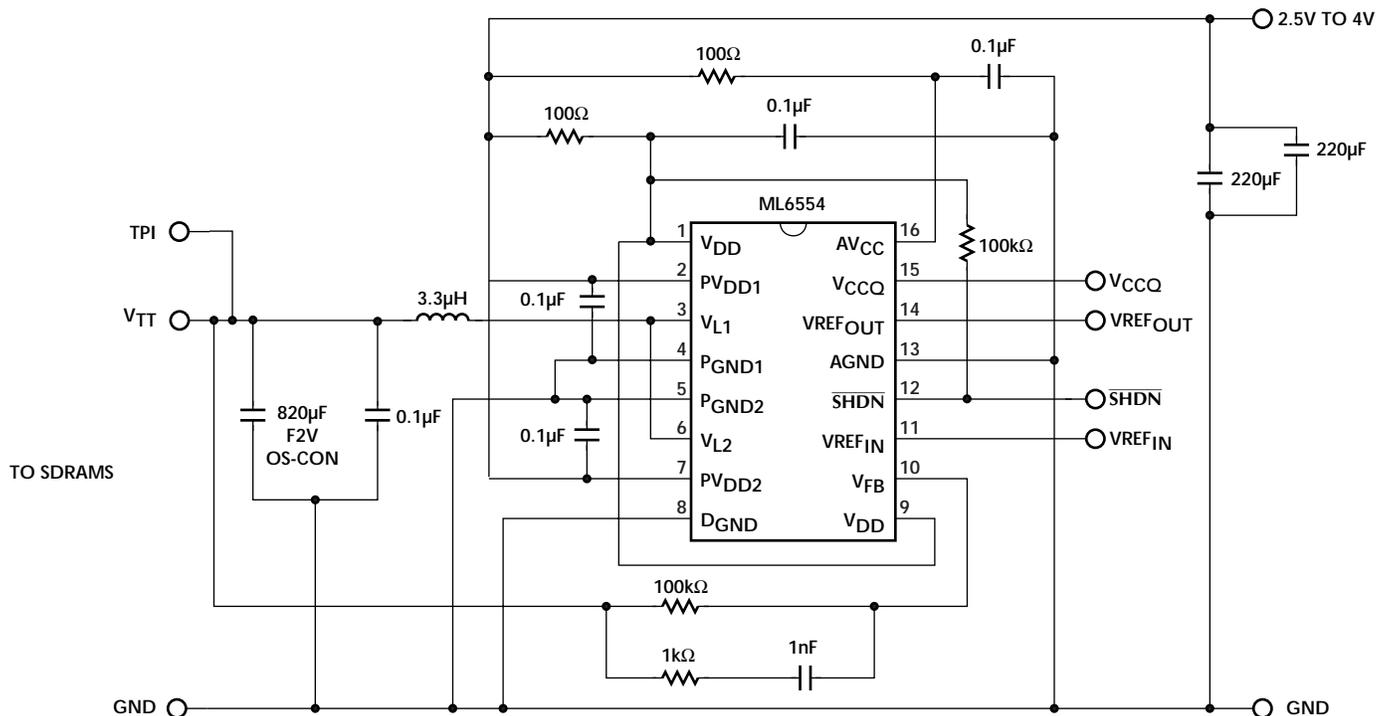
Figure 9. Micro Linear ML6554 Evaluation Board Schematic
