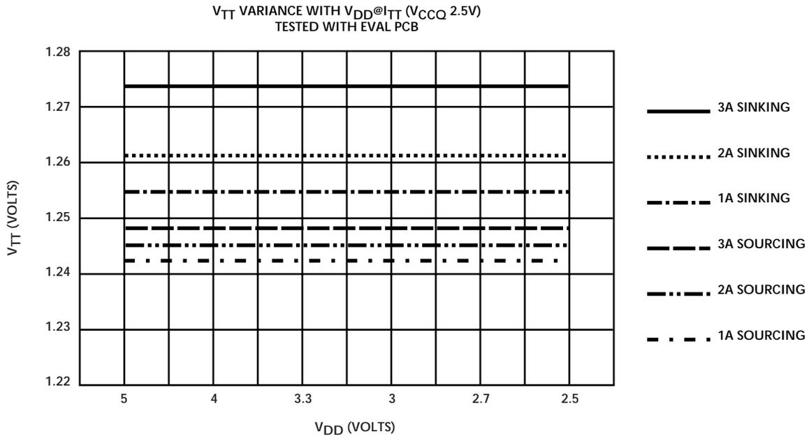
Figure 14. V<sub>TT</sub> Performance for SSTL\_2 Bus
