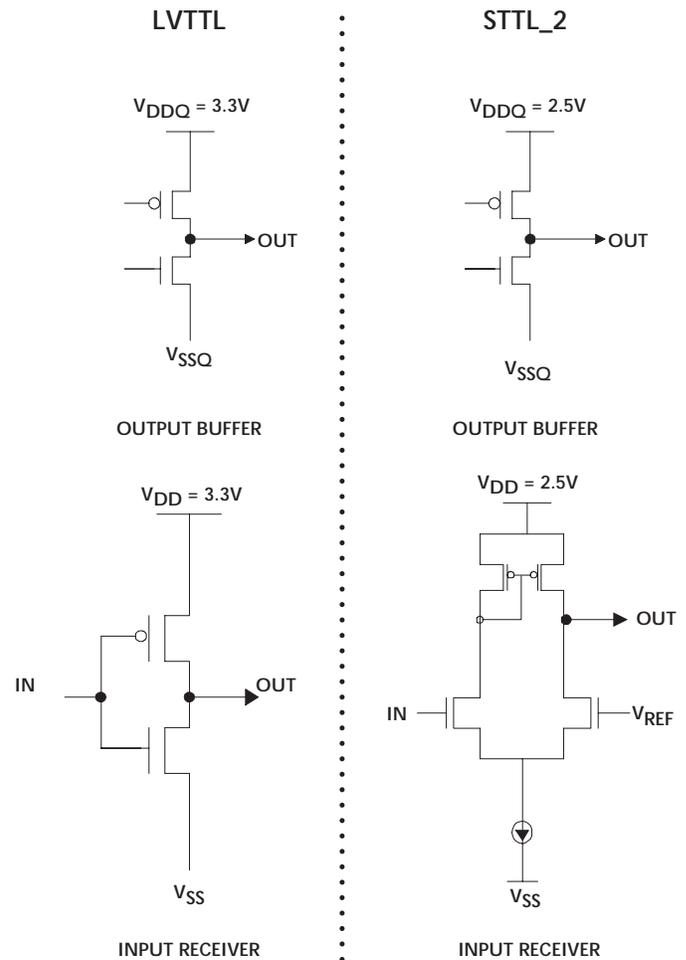
Figure 2. Comparison of LVTTTL and SSTL\_2 Drivers and Receivers
