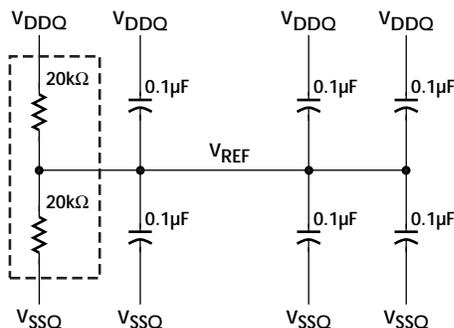
Figure 5.  $V_{REF}$  Network for PC266 DDR SDRAM
